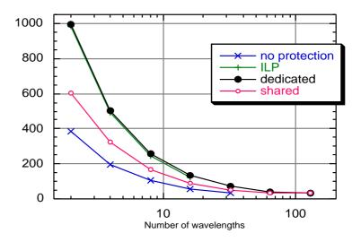
Node-disjoint protection is similar to link-disjoint since nodal degree is less or equal 3
